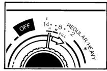
**LOWER WATER LEVELS.** Setting the washer to fill with less water also sets it for shorter wash time.
